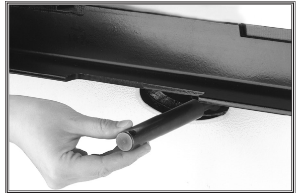
Figure 26. Installing the splitter shaft.
